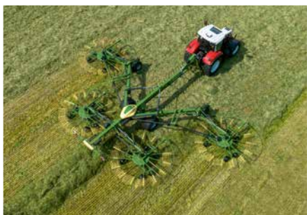
Swadro TC 1570 Pro Four-rotor rake centre delivery Variable working widths from 11.00 m to 15.70 m
