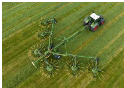
Swadro TC 2000 Pro Six-rotor rake centre delivery Variable working widths from 10.00 m to 19.00 m
