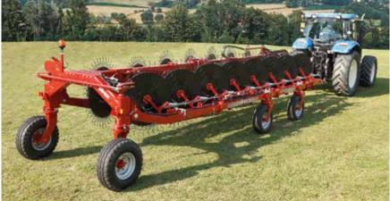
TRANSPORT POSITION Machine in transport position on the road
