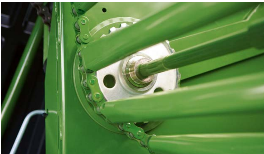
One of the guide rollers and the chain-and-slat elevator (variable chamber model)
